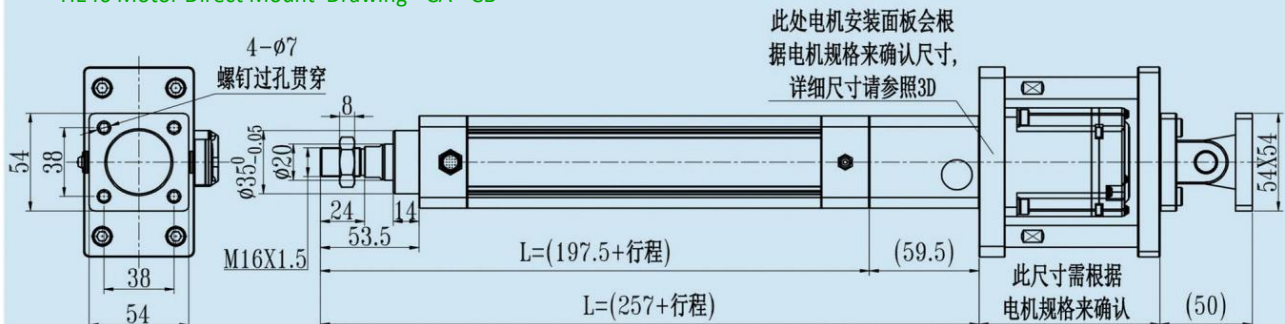
HE40电机直接安装外形图-双耳环安装-CA-CB HE40 Motor Direct Mount Drawing - CA - CB
